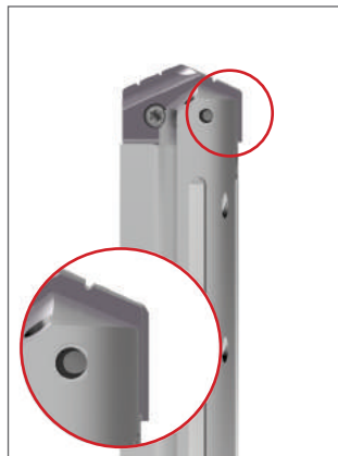
Adjust insert position.
